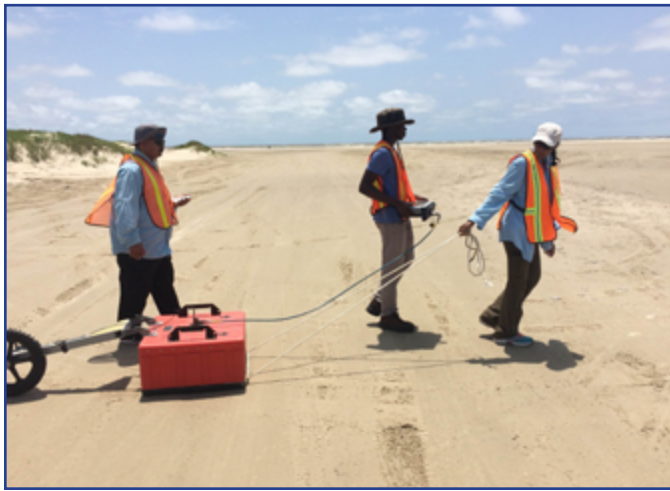
Figure 3: Dr. Shuhab Khan (far left) and students conducting GPR survey, San Luis Pass, TX.
